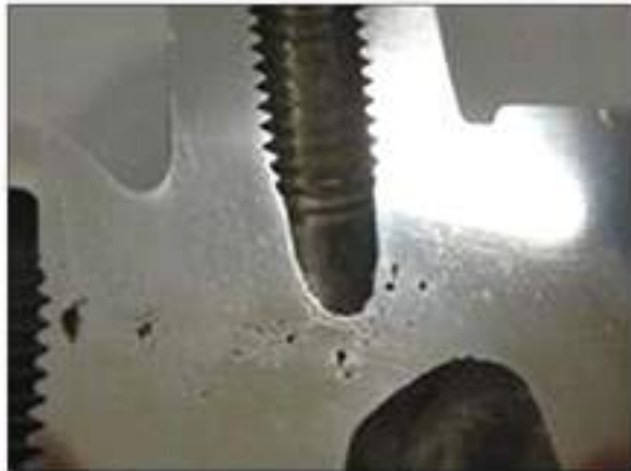
Casting without use of Jet Cool System (Porosity occurs near the threads)
